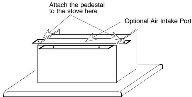
Lift the stove onto the pedestal. Line up the threaded bolt holes in the bottom of the stove with the two holes in the tabs that stick out of the side of the pedestal. Using an open-end or socket wrench, fasten the pedestal to the stove with the supplied bolts and washers.
