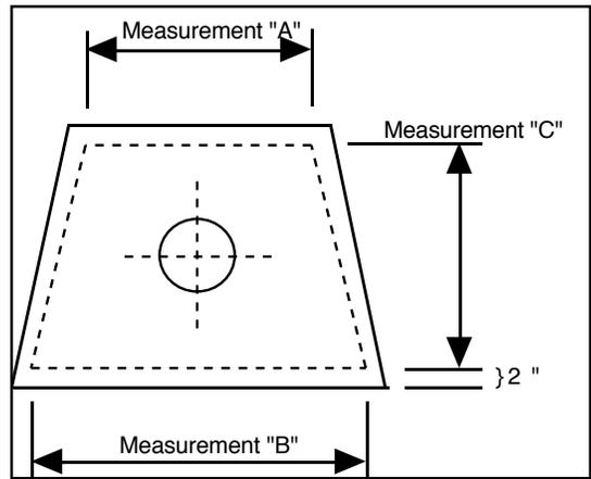
5. Bend the sheet metal as indicated on the template at a 45 degree angle on each side after cutting the sheet metal (This 2" lip will allow you to screw this plate into the smoke chamber inside your fireplace). The 2" lip with the 1/4" diameter holes will allow you to screw the plate to the firebox walls.
