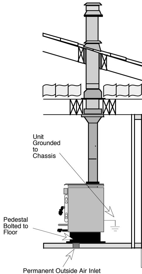
**CAUTION:** The structural integrity of the mobile home floor, wall, ceiling and roof must be maintained.
