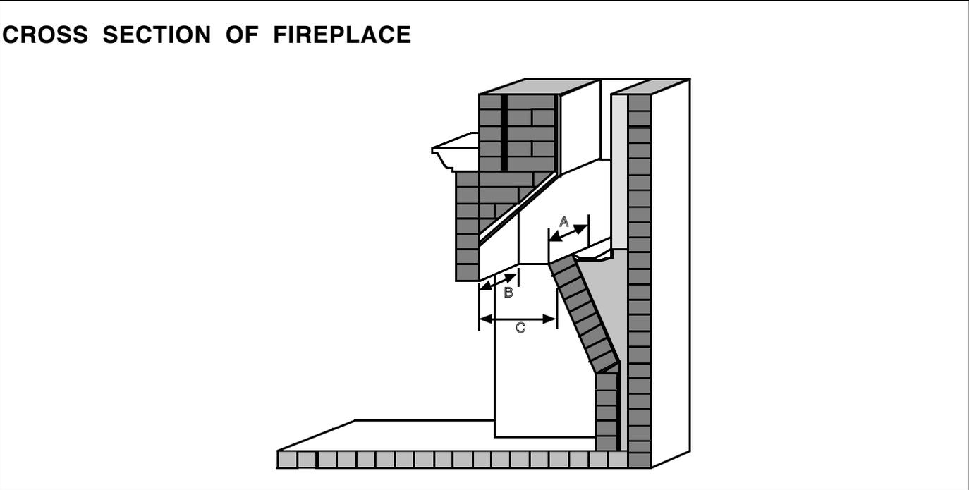
Your template should resemble the drawing on the next page with the dotted lines indicating your initial measurements and the solid line indicating the additional 2". You will use this template to cut a piece of sheet metal (minimum 24 gauge) to install in your smoke chamber.
