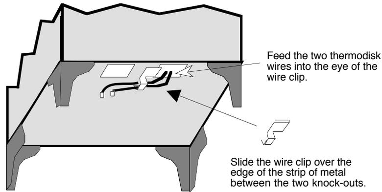
**NOTE:** The wires coming from the thermodisk assembly must not have too much slack – these wires pass near the firebox and can cause a short if the slack is not taken in and held in place with the wire clip. Do not pull so hard on the wires that you dislodge the thermodisk housing from its location.
