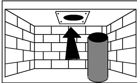
11. Once the insert is in position and leveled, connect the 6" liner to the unit and secure it with sheet metal screws through the holes in the flue collar.
