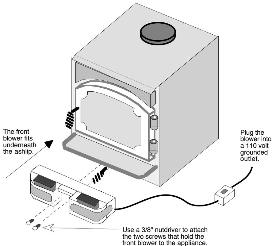
1. Remove the two screws below the ashlip with a 3/8" nutdriver.
