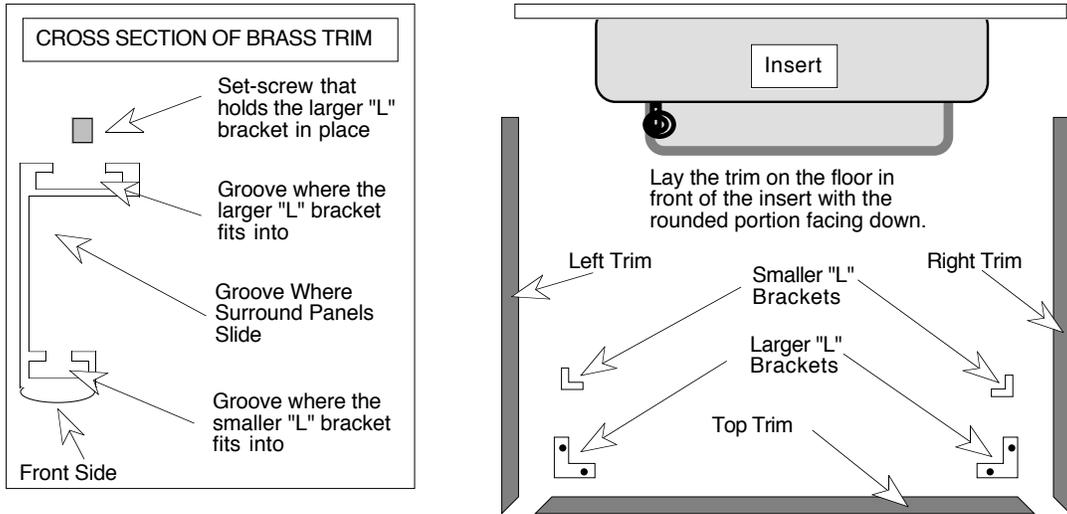
2. Insert a large and small "L" bracket leg into the groove in the 45° cut end of each side piece. Slide the other leg of each "L" bracket into the groove in each end of the top piece.
