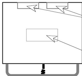
After the precise location of the stove is determined, the outside air boot or pedestal with outside air should be installed prior to installing the stove. Follow the directions included with the outside air boot or pedestal. Make sure to remove the correct knock-out for the outside air option. See the illustration to the left.
