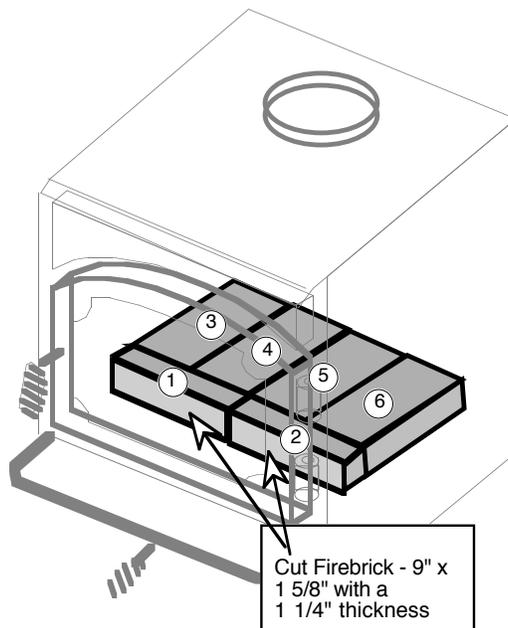
5. To replace the floor firebricks, follow these directions in reverse order, placing the bricks snug against the firebricks lining the side of the firebox.
