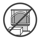
o It is imperative that control compartments, screens, or circulating air passageways of the heater be kept clean and free of obstructions. These areas provide the air necessary for safe operation.
