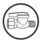
Instruct everyone in the house how to shut gas off to the appliance and at the gas main shutoff valve. The gas main shutoff valve is usually next to the gas meter or propane tank and requires a wrench to shut off.
