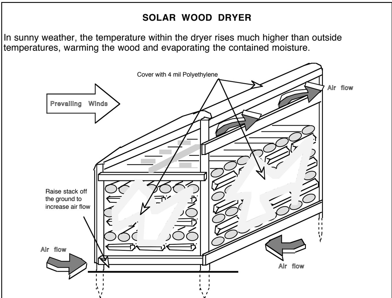
Many arrangements for plastic covering are possible. Thin 2 millimeter, clear polyethylene sheeting sold for drop cloths or garden mulching is not recommended because it is easily torn. The 4 millimeter thickness is more satisfactory and less costly than 6 millimeter. Any clear polyethylene deteriorates badly after a few months of exposure to full sunlight, so the stack may have to be re-roofed to remain dry over winter.
