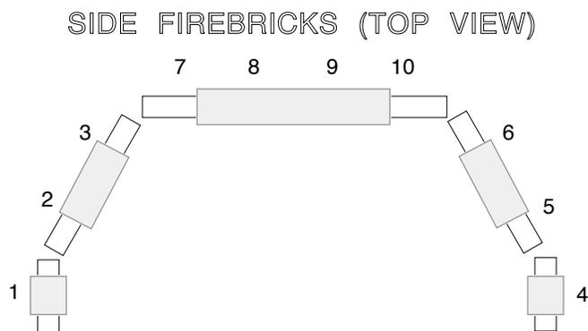
4. When replacing any of the side firebricks, use firebrick available from your dealer. The dimensions of the side firebricks are 1 1/4" thick, 4 1/2" wide, and 9" long. The left side firebrick located in front (Brick #1) has a hole drilled in it for gas line installation. If this firebrick is damaged and needs to be replaced, make sure to specify this when ordering a replacement firebrick.
