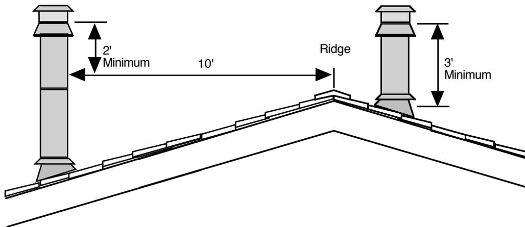
2. **CHIMNEY SIZE:** Your Fireplace Xtrordinair is tested with 8" ID metal chimney and 12" x 12" clay flue liner. The use of any other size is not recommended and is likely to cause problems in achieving proper draft.
